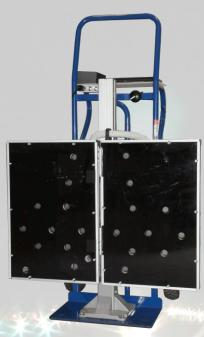
SMF/Fix is a stop-and-go real-time photometric measurement system for AGL equipment, designed, developed and manufactured by ARGOS in order to perform the measurement of the airfield lights along runways and taxiways without the requirement of a vehicle.
